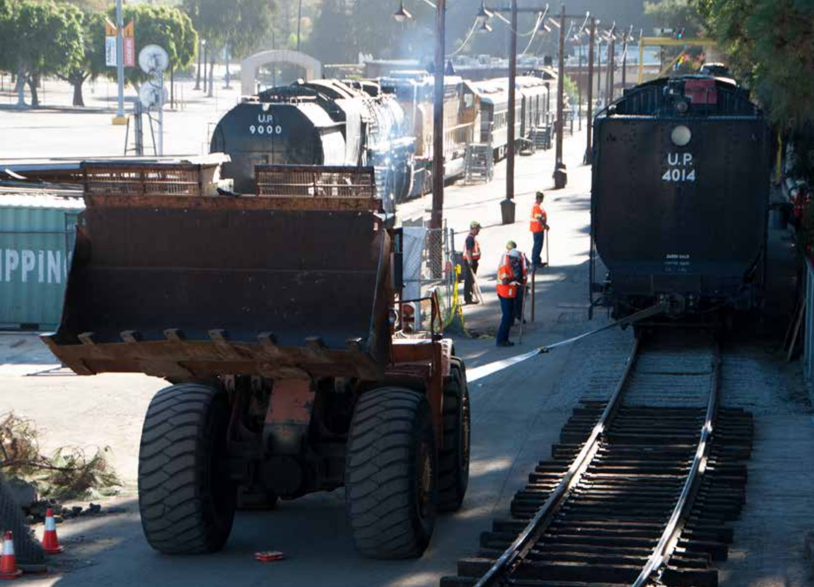
Nov. 13, 2013, will always be known as the day when No. 4014 started down the road to restoration. A front-end loader tied to the tender coupler gently tugs the dead locomotive backward from its display site at the Los Angeles County Fairgrounds and the Rail Giants Museum.
