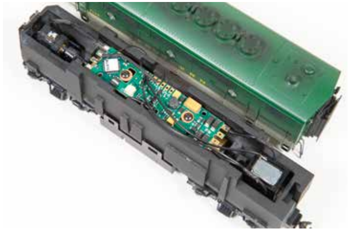
Turn to page 14 and follow along as Larry Puckett demonstrates how to install sound decoders into a pair of older HO scale Electro-Motive Division F units. Photo by Larry Puckett
