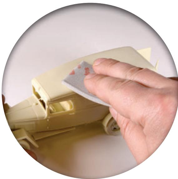
First, remove the excess putty with 200-grit sandpaper. Focus on the filled spot to prevent damage to your piece or removing nearby detail.
