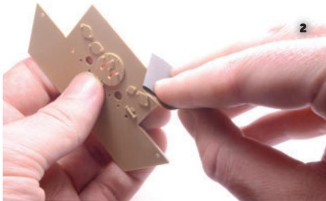
2. Go over the whole area with fine sandpaper or a sanding stick. If the part is metal, use a file to remove excess material.
