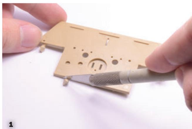
1. Remove the burr with a hobby knife. Try to be very precise and remember that the knives cut best when you use a slicing motion, not just pressure.
