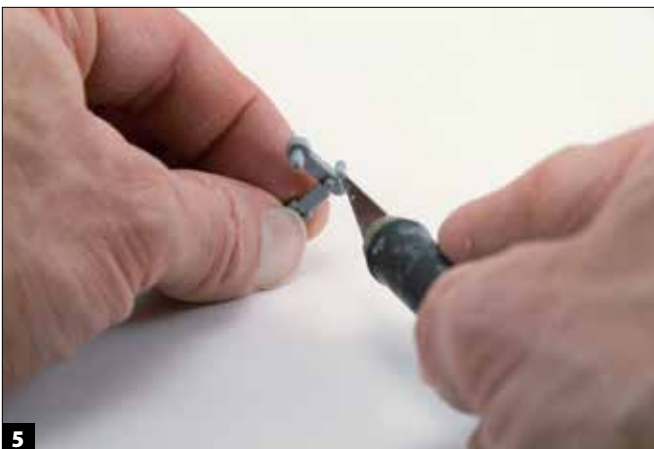
5 Each of the suspension units had a mold seam that I eliminated by first scraping a no. 11 blade along it, keeping the edge perpendicular to the surface.
