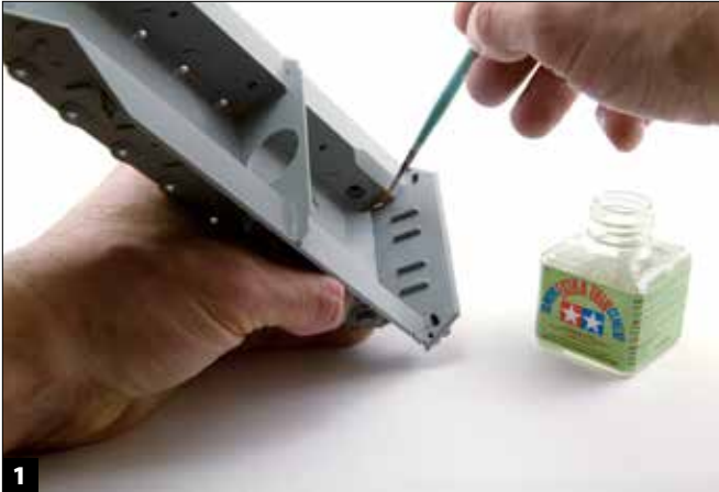
1 The Leopard's hull features separate bottom and side panels with an internal brace. Applying liquid cement from the inside minimizes the opportunities for glue to mar external surfaces.
