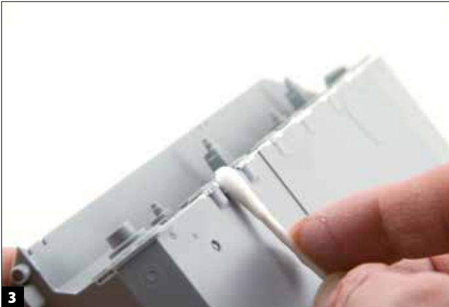
3 The water-based putty is easily smoothed with a damp cotton swab, which virtually eliminates the need for sanding.
