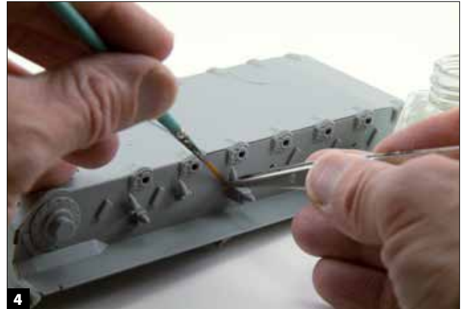
4 I trimmed the Leopard's springs off close with side cutters. A sanding stick makes quick work of the sprue attachment points and mold seams of the springs. Tweezers make it easy to handle small parts. Here, I hold a spring into place and flow liquid cement into the join.
