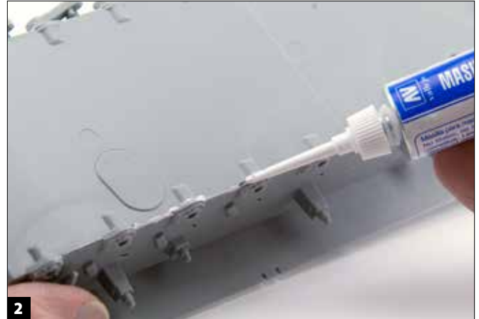
2 To fill minor gaps around the lower hull, I squeezed in a little Vallejo plastic putty. The pointed applicator works much like a caulking gun and is ideal for fine lines.
