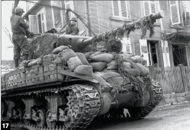
17 The sandbag racks on this tank are less complicated than those seen on the M4 in photo 16. Racks were made in unit shops, so they varied quite a bit in design.
