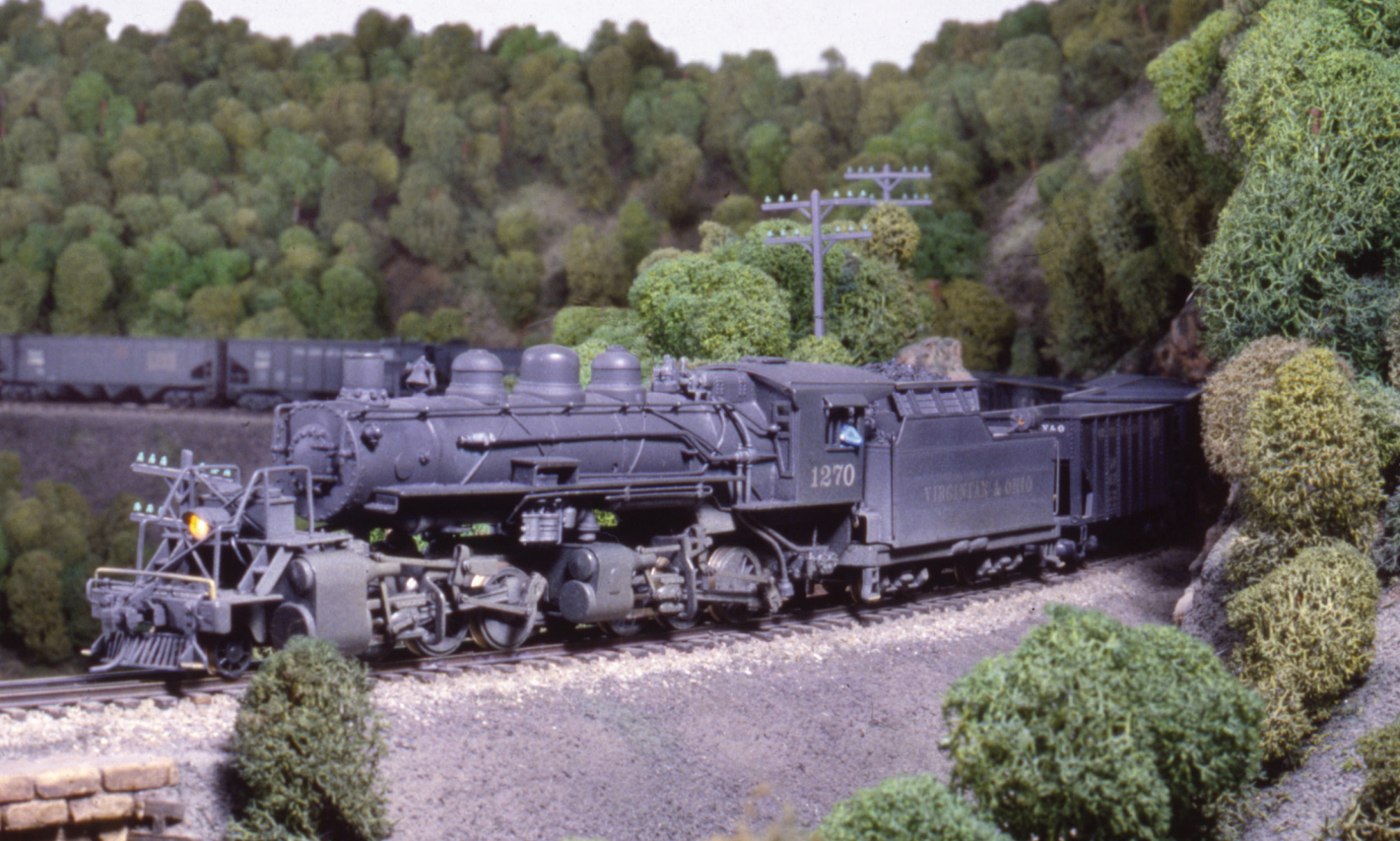
A Pacific Fast Mail 2-6-6-0 Sierra Mallet-type articulated with the trailing truck removed looked rugged enough for Appalachian service with extended coal-bunker sides. It performed well in coal shifter and helper service. But no. 1270 (originally 170) was the only one on the V&O roster. Here it makes the official last steam run in December 1980.
