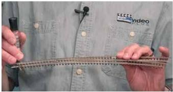
Are locomotives or cars shorting on the sides of the points or frog of turnouts? Put some clear (or brown) nail polish on the offending rail. Nail polish is built to be tough. It'll stand up to train wheels bumping it for a long, long time. If the polish wears off, just apply some more. (Episode 13)
