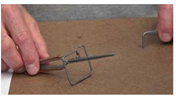
**You usually need three** hands when soldering at your workbench. But not if you buy special self-closing soldering tweezers. This tool will keep your wires steady, letting you hold the soldering iron and solder. The tweezers are also referred to as cross locking, and are available with or without a stand from most electronics suppliers. (Episode 45)
