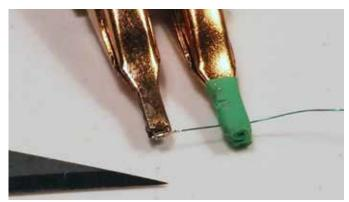
If regular soldering is difficult, soldering wire to surfacemount light-emitting diodes (LEDs) is really tedious. Make it easier on yourself by investing in an LED/wire holding tool (no. NT301) from ngineering.com. It holds even nano LEDs and wire in place so you can simply touch the soldering iron to the LED and wire to secure it. (Episode 45)
