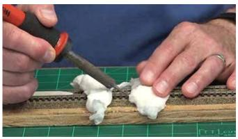
**When soldering,** the idea is to do it quickly so you don't damage the parts. But sometimes stuff just doesn't want to be soldered quickly. What you need is a "heat sink." And the quickest, cheapest one you can possibly use is a piece of wet facial tissue. Plunk a piece on both sides of where the solder will be applied, or on the wires, and it'll keep that heat from doing any damage. (Episode 53)
